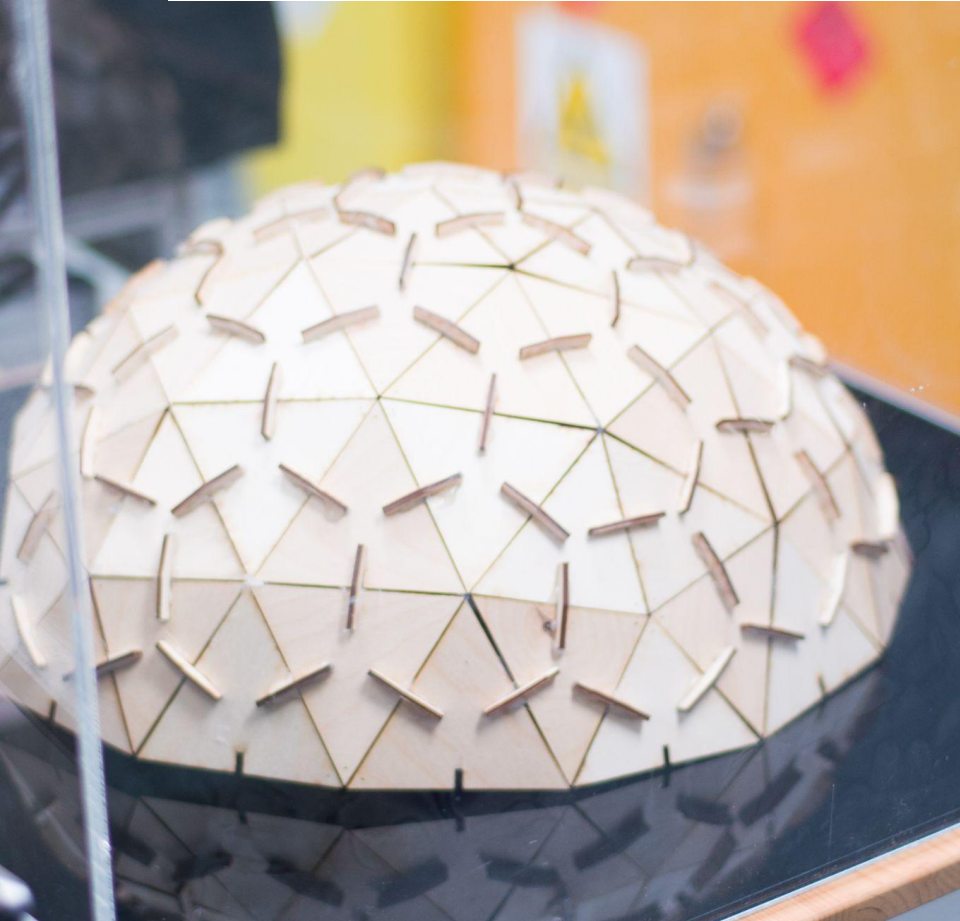
Prototype of a fungal building by Dr. Neil Phillips. Geodesie of a dome is formed by two different sized triangles.
