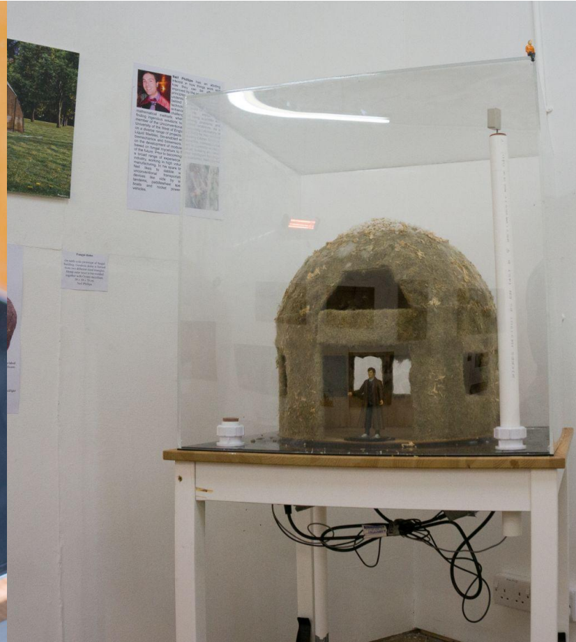
Prototype of a fungal building by Dr. Neil Phillips. Geodesie of a dome is formed by two different sized triangles.
